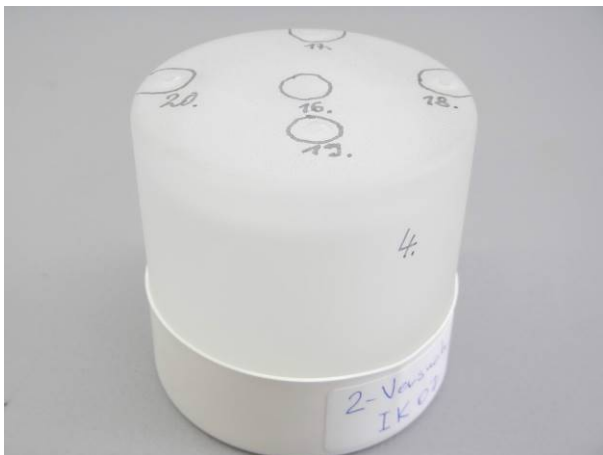
Picture 5 Sample No.2 with visible chips on the material and no cracks on the surface after the impact test IK07 (Impacts S16 – S20)
